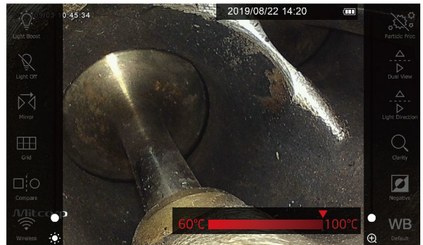
100°C resistance warning & auto shut down protection
