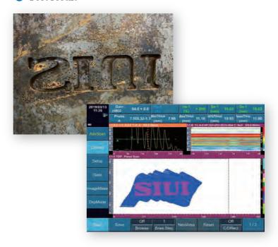
Scanning on pipe (wall thickness 4mm)
